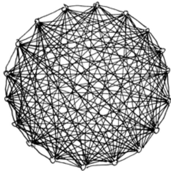
*Fig. 6 A completely-connected set of nodes.*
